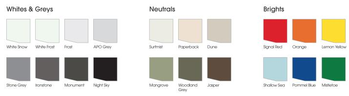
This colour chart is to be used as a guide only. The final glass colour may differ from these printed colours. The natural green tone of standard glass can affect light colours and can be minimised by specifying VFloat™ SuperClear low iron glass.
