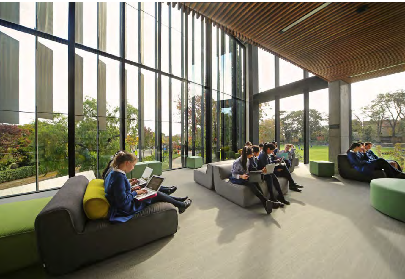
North-facing informal learning spaces are deftly screened to assist the quality of experience, privacy, and solar loads.
