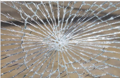
VLam, if broken the glass is bonded to an interlayer.
