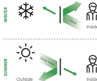
The U-Value explains the insulation level of your glass. The lower the U-Value, the better the glass is at keeping your home a comfortable temperature all year round.
