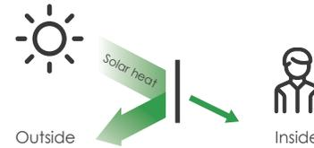
SHGC measures how much solar heat passes through the glass, the lower the SHGC the better the glass is at keeping unwanted heat out – keeping you cooler in summer!
