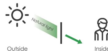
The VLT value shows how much light the glass is allowing into your space. The higher the VLT, the more natural light is being transmitted through the windows.
