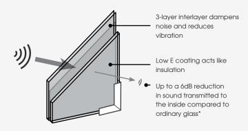
VLam™ Hush uses a special interlayer that targets sounds through the frequency range with an enhanced effect on higher frequencies - the most sensitive range of human hearing.
