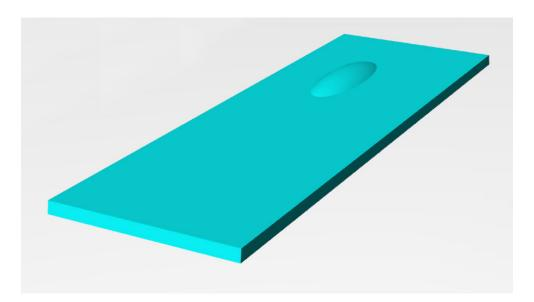
Local distortion refers to an undulation forming in one part of the glass only. It can be of any shape.
