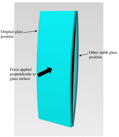
The picture above shows the two stable positions for a sheet of toughened glass with a bi-stable characteristic. A force applied in the direction of the arrow will cause the panel to pop to the other stable shape.
